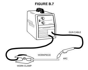
When no more welding is to be done, close valve on gas cylinder (if used), momentarily operate gun trigger to release gas pressure, and turn off the Handymig 170i.
